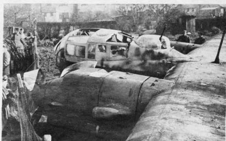
Rounded nose of Do-217M1 sets it apart from other models. This late Nazi bomber was shot down during desperate raids on London.
